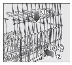
■ Press the insert downwards ① and press the catch inwards at the same time ②.
